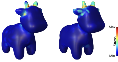
Figure 8: Distribution of maximum stresses computed for a fully solid model. Estimated stress (left) is an approximation of the ground truth (right), obtained with a lower computational cost.
